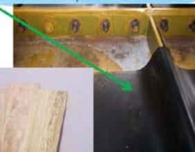
Composite panels (to shield from radiation from the wall)
