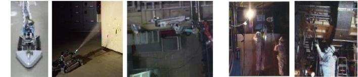
Developed by ATOX, Ltd. Remote handled decontamination machines (for floors, and low and medium height places).
