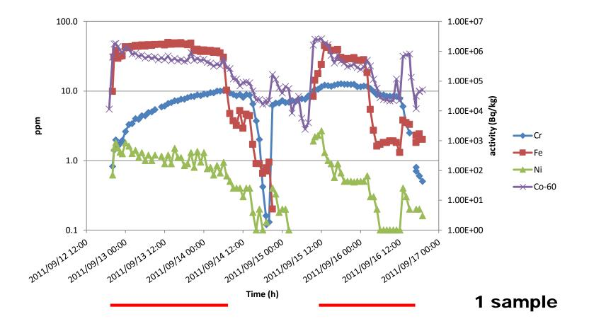
Average concentration of water going through ion exchange resin.
