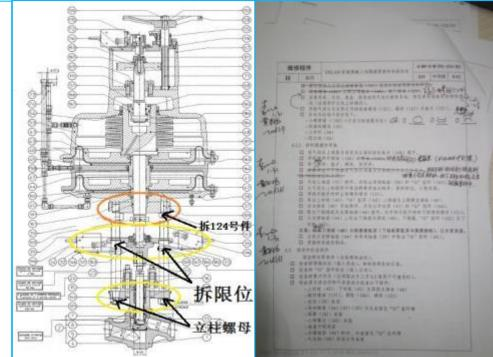
Taking H203 outage as an example, 4man.mSv was reduced by the optimization of the disassembly of five pneumatic heads in high-dose area.
