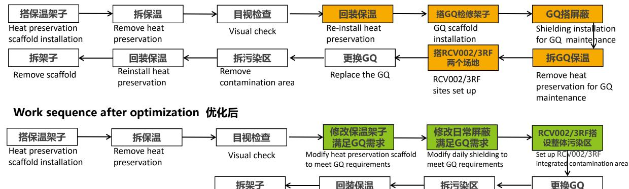
Contamination area One time of shielding construction and removal + one time of heat preservation removal and installation, 80% of scaffold erection time and 40% of site erection time are reduced by this optimization.
