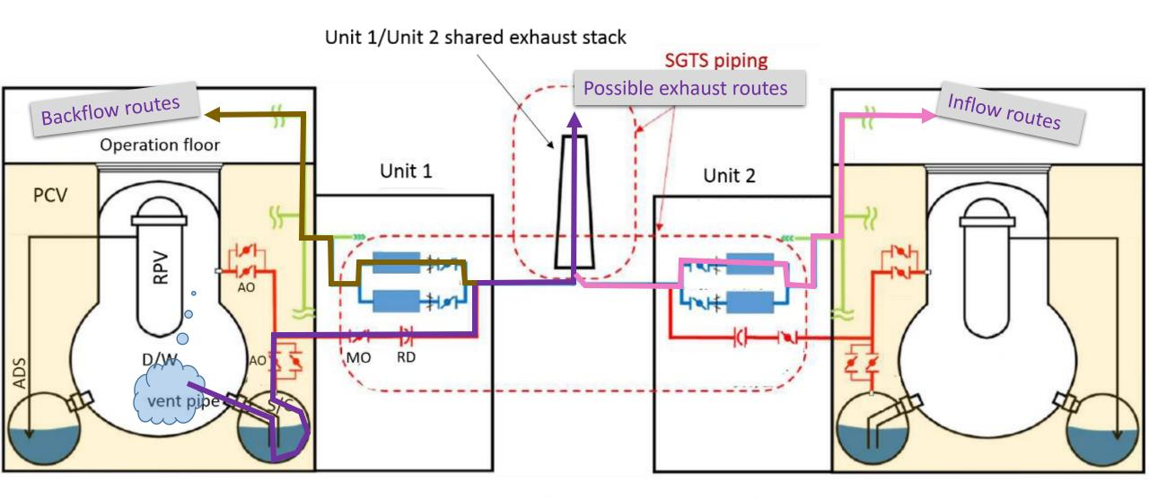
The contamination of the SGTS piping systems of Units 1 and 2 was confirmed by the results of the site investigation and the results of the JAEA analysis.
