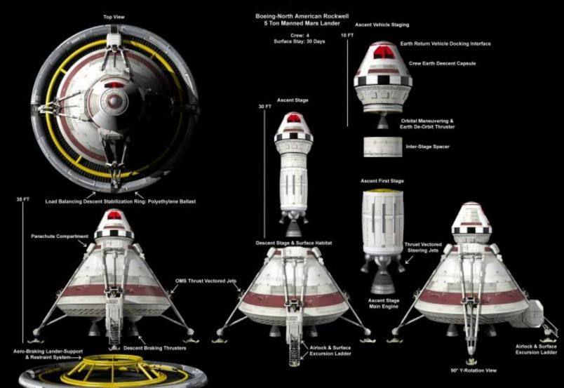
kero-Braking/Reentry Heat Shield
