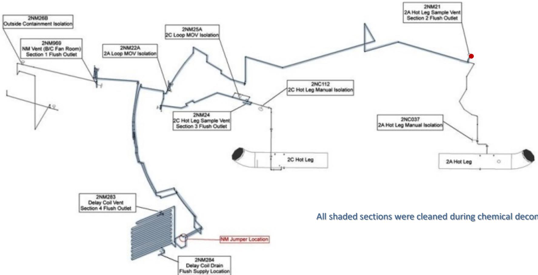
All shaded sections were cleaned during chemical decon.
