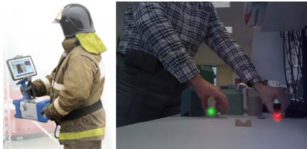
Example of image obtained from the camera in a 1 s frame - 3.7 MBq Am-241 source in red and 1.7 MBq Co-57 in green.
