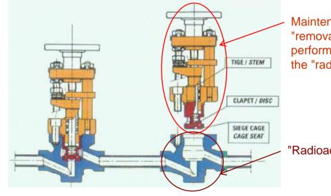
Maintenance on "removable part" performed away from the "radioactive part"
