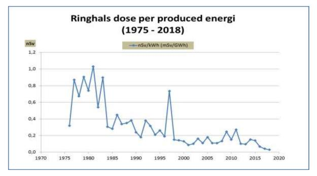
Ringhals availability on grid has improved as well as decreasing CRE have resulted in a level of 30  $\mu$ Sv per produced GWh.
